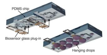
Fig. 10 Design of the droplet array microfluidic device with enzyme-modified electrodes.<sup>73</sup> Reproduced from Springer Nature ©2016.
