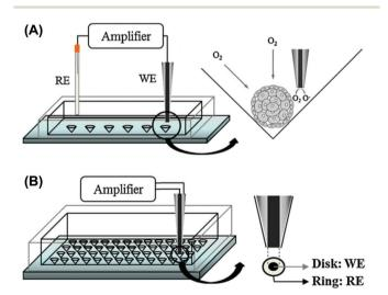
Fig. 3 Electrochemical detection of  $O_2$  consumption by 3D cultured cells using SECM.<sup>14</sup> (A) Conventional SECM system, working (WE) and reference (RE) electrodes are inserted into a solution, and 3D cultured cells are trapped in a microwell. (B) Probe devices containing both working (WE) and reference electrodes (RE) for simplifying the detection procedure. Reproduced with permission from Elsevier ©2012.
