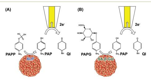
Fig. 5 Schemes of electrochemical detection for (A) endogenous ALP and (B) SA-β-Gal.
