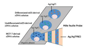
Fig. 7 Mille-feuille probe containing the lamination of the aqueous and organic phases under voltage control for simultaneous detection of multiple cDNAs collected with the mille-feuille probe.<sup>37</sup> Reproduced with permission from Springer ©2017.
