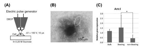
Fig. 6 mRNA collection from cells using the DBCP.<sup>32</sup> (A) General outline. (B) Phase contrast image of the 3D cultured ES cells differentiated into cardiomyocytes. A dashed line indicates the beating area. (C) Relative gene expression of Actc1 in the cells at the beating area and at the nonbeating area. Reproduced with permission from Springer ©2014.
