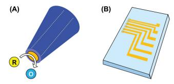
Fig. 2 Electrochemical probe (A) and chip (B) devices.
