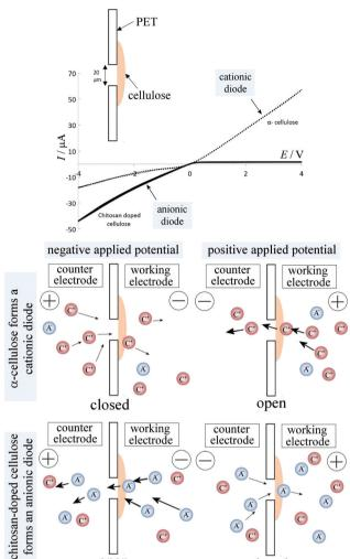
Fig. 5 Cyclic voltammetry (scan rate: 20 mV s $^{-1}$ ) of  $\alpha$ -cellulose only films (dotted line) and chitosan-doped cellulose films (black solid line) on a 20  $\mu$ m diameter microhole in a PET sheet in 50 mM NaCl on both sides of the membrane. The schematic drawing shows the four mechanistic cases of a cationic diode and an anionic diode under positive potential and negative potential polarisation, respectively.
