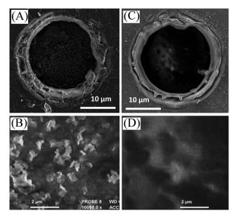
Fig. 2 Scanning electron micrograph (SEM) images for (A, B) a cellulose film deposit and (C, D) a chitosan-doped cellulose film deposit on a 20  $\mu$ m diameter microhole in a PET film.
