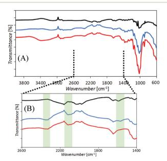
Fig. 3 (A, B) FTIR spectra of chitosan (black line); cellulose (red line); and cellulose–chitosan blend (blue line) bulk films cast for analysis. Signals unique to both cellulose ( $2400-2300~{\rm cm}^{-1}$  and  $2160-2040~{\rm cm}^{-1}$ ) and chitosan ( $1600-1550~{\rm cm}^{-1}$ , attributable to N–H bonds) are present in the co-deposited films, confirming the presence of both polymers.
