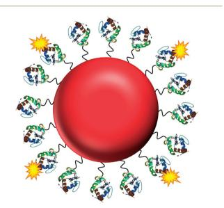
Fig. 1 The NO nanobiosensor: cytochrome c (structure obtained from the Protein Data Bank – PDB ID 1HRC)<sup>28</sup> fluorescently tagged with Alexa Fluor 488 (yellow) assembled onto a gold nanoparticle (red) surface via a SPDP linker (black).
