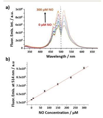
Fig. 2 (a) Fluorescence excitation (left;  $\lambda_{ems}$  = 514 nm) and emission (right;  $\lambda_{\rm exc}$  = 492 nm) spectra of the NO nanobiosensor in the presence of increasing concentrations of NO (from 0 to 300  $\mu$ M). (b) Calibration curve of the NO nanobiosensor obtained from the fluorescence emission intensity at 514 nm as a function of the concentrations of NO; error bars show the mean error of 3 replicates. y = 1217x + 584141.
