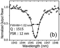
Fig. 2 (a) SEM image of a silicon ring resonator on a silicon-on-insulator (SOI) platform. (b) Corresponding transmittance spectrum: experimental points (symbols) and Lorentzian fit (solid line). Adapted with permission from S. Lin et al., Nano Lett., 2010, 10, 2408-2411 (ref. 27). Copyright 2010 American Chemical Society.
