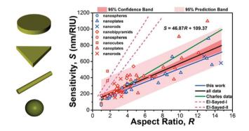
Fig. 6 Bulk sensitivity (in units of nm RIU<sup>-1</sup>) of different types of plasmonic nanostructures supporting LSP resonances with different aspect ratios. Different symbols correspond to different structures. Reproduced with permission from A. U. Khan et al., J. Phys. Chem. C, 2016, 120, 19353-19364 (ref. 59). Copyright 2016 American Chemical Society. For the meaning of the different colours, lines and shades the reader is referred to ref. 59.
