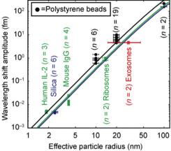
Fig. 12 State of the art for single particle detection using a purely photonic WGM resonator. Wavelength shift as a function of the particle radius for different types of synthetic and biological nanoparticles: human interleukin-2 molecules, SiO<sub>2</sub> beads, mouse immunoglobulin, human ribosomes, mouse exosomes, and polystyrene nanobeads. The solid lines are calculated from the reactive sensing principle (eqn (6)). Reproduced from ref. 121
