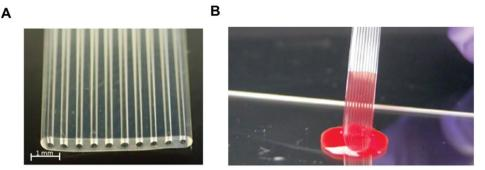
Fig. 3 Microcapillary film (MCF) platform for a sandwich immunoassay using whole blood samples without sample treatment. (A) Microphotograph of 10-bore MCF containing 200 µm internal diameter microcapillaries. (B) 'Lab-on-a-stick' showing the loading of a blood sample by capillary action based on a fluoropolymer MCF coated with hydrophilic polyvinyl alcohol.
