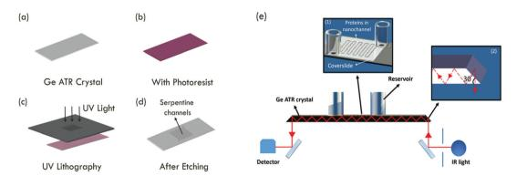
Fig. 1 (a)-(d) Fabrication scheme of serpentine nanochannels on Ge ATR crystals. (e) Schematic set up for ATR-IR spectroscopy on a Ge nanochannels nel device. Inset (1) shows an enlarged image of the nanochannel region. Inset (2) shows chip edges ground to 30° angle to facilitate 60° angle of
