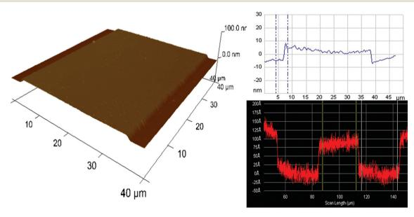
Fig. 2 AFM 3D profile showing a section of one of the post regions in the 10 nm deep nanochannel. Top right is the height measurement obtained using AFM and the bottom right image is from surface profiler measurements, showing the height of the nanochannels of  $\sim$ 10 nm.
