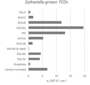
Comparison of conductivities of epitaxially-grown monocrystalline transparent conducting oxides, as compared with current conventional carbon-based TCMs. The full data set with author references is given in Table 1
