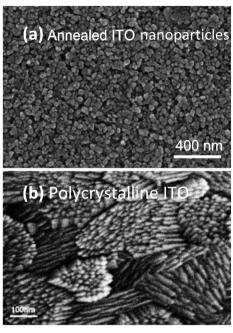
Fig. 5 Scanning electron micrographs from (a) an ITO thin film inkjetprinted from 25 nm nanoparticles and annealed at 450 °C, 28 and; (b) conventional DC magnetron sputtered polycrystalline ITO film deposited at 200  $^{\circ}\text{C}.^{27}$ Adapted with permission from Jeong et al. and Betz et al.<sup>27,28</sup> Copyright (a) 2010 and (b) 2006 Elsevier.
