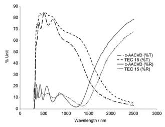
Fig. 13 Optical transmittance (%T) and reflectance (%R) spectra of SnO<sub>2</sub>:F lab-grown by combinatorial aerosol-assisted chemical vapour deposition (c-AACVD) as compared with an industrial SnO2:F product (TEC 15, Pilkington NSG). Adapted with permission from Bhachu et al. 37 Copyright 2011 Wilev
