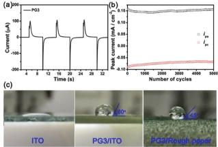
Fig. 4 (a) Chronoamperometry for PG3 with a 5 s delay for each potential (-0.1 V and +0.8 V). (b) Stability of a 600 nm thick PG3 film cycled 5000 times with a scan rate of 100 mV  $s^{-1}$  in 0.1 M TBAPF<sub>6</sub>/ACN: the change in the anodic  $(\Box)$  and cathodic  $(\bigcirc)$  peak currents as a function of number of cycles. (c) Photographs of the water droplet volume of 10 µL on the surface of ITO, PG3/ITO and PG3/rough paper, respectively.
