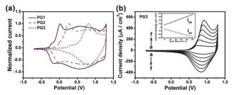
**Fig. 2** (a) Single scan cyclic voltammetry of different films at 100 mV s<sup>-1</sup> in 0.1 M TBAPF<sub>6</sub>/ACN: PG1 (black, solid line), PG2 (red, dashed line), and PG3 (blue, short dashed line). (b) Scan rate dependence of the PG3 film in 0.1 M TBAPF<sub>6</sub>/ACN at (a) 50, (b) 100, (c) 150, (d) 200, (e) 250 and (f) 300 mV s<sup>-1</sup> (inset is the plot of scan rate with anodic ( $i_{pa}$ ) and cathodic ( $i_{pc}$ ) peak currents).
