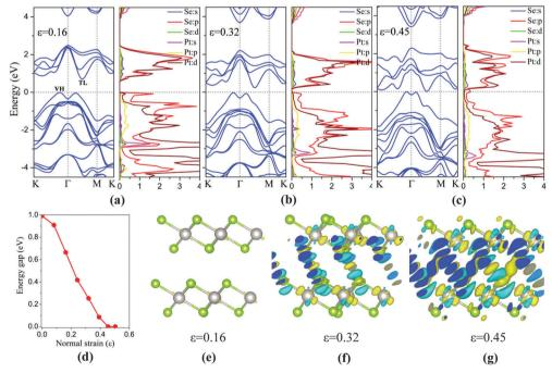
Fig. 6 (a-c) Computed band structure and partial densities of states of  $PtSe_2$  bilayer under three different VCS values, with the corresponding differential charge densities plotted in (e-g). The Fermi level is located at 0 eV. (d) Band gap of bilayer *versus* normal strain.
