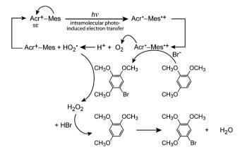
**Fig. 12** Schematic representation of the photocatalytic bromination of 1,2,4-trimethoxybenzene (TMB) with 9-mesityl-10-methylacridinium (Acr<sup>+</sup>–Mes) as a catalyst. SE: Singlet excited state.
