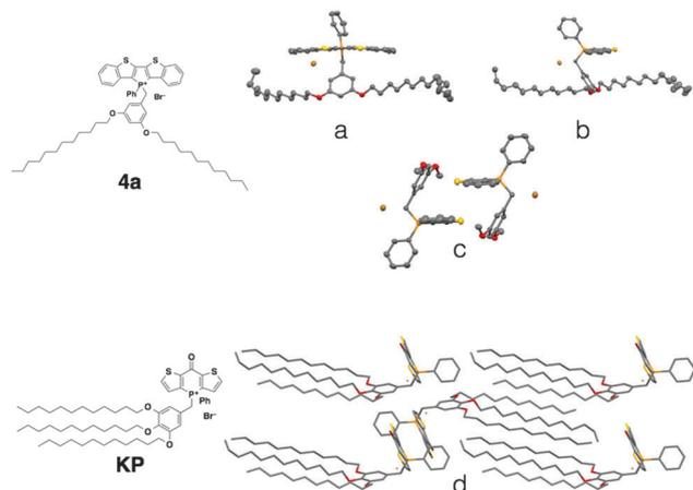
Fig. 11 Single crystal XRD data of phosphole-lipid (**4a**) and phosphinine-lipid (**KP**). (a) and (b) solid-state structures of **4a** as monomers; (c) the intermolecular packing of **4a** (dodecyl chains are truncated for clarity); (d) solid-state packing of **KP**.<sup>9</sup>
