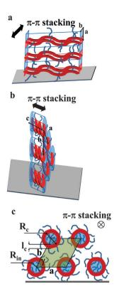
Fig. 6 Models schematically depicting the layer-like structure of thin films of  $P_a$  (a) and  $T_a$  (b). The polymer backbone is represented in red while the film surface is the gray parallelogram. (c) The view along the helical axis represents notations used in eqn (7) and (8). The inner part of the helices is colored in blue, the area of the pseudo-hexagonal unit cell external to the helices is colored in green (c)
