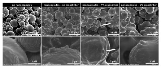
Fig. 4 SEM images of sliced sections of Porous-PA13 monoliths incubated with blank nanocapsules with 0-2% crosslinker showed penetration of the nanocapsules (arrows) into the polymer network. Scale bar top row 10 µm (2000×) and bottom row 2 µm (3500×).
