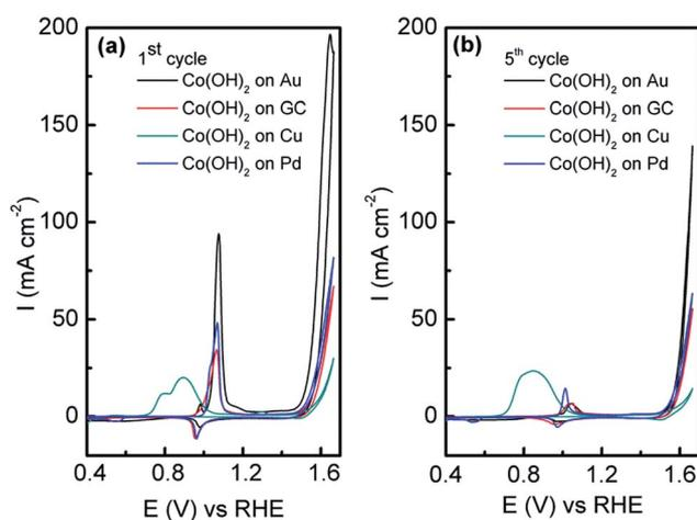
Fig. 5 Cyclic voltammograms recorded at Co(OH)<sub>2</sub> electrodeposited on Au and GC electrodes and an unmodified Au electrode in 1 M NaOH recorded at 50 mV s<sup>-1</sup> showing (a) the first cycle and (b) the fifth cycle.
