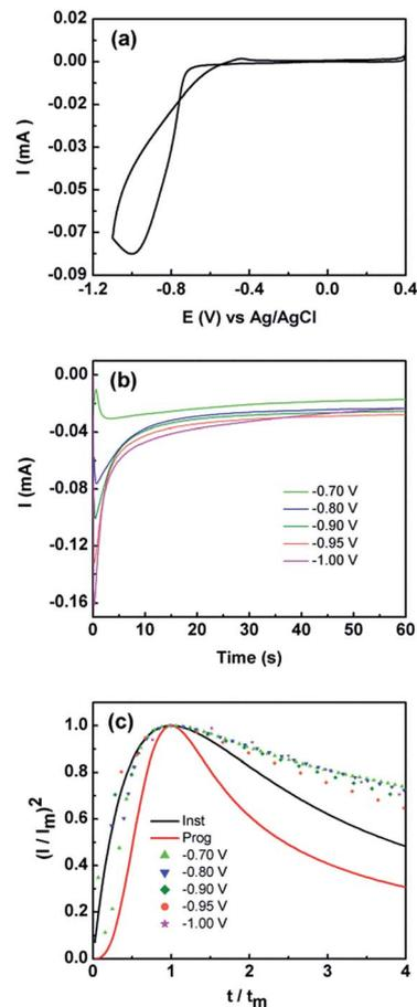
Fig. 1 (a) Cyclic voltammogram obtained at  $50 \text{ mV s}^{-1}$  at a Au electrode in 10 mM  $\text{Co}(\text{NO}_3)_2 \cdot 6\text{H}_2\text{O}$  solution (b) current–time curves obtained at different applied potentials and (c) non-dimensional plots of  $(I/I_m)^2$  vs.  $t/t_m$  for the electrodeposition of  $\text{Co}(\text{OH})_2$ . Overlaid are the theoretical curves calculated using eqn (3) and (4) for progressive (—) and instantaneous (---) nucleation and diffusion limited growth.
