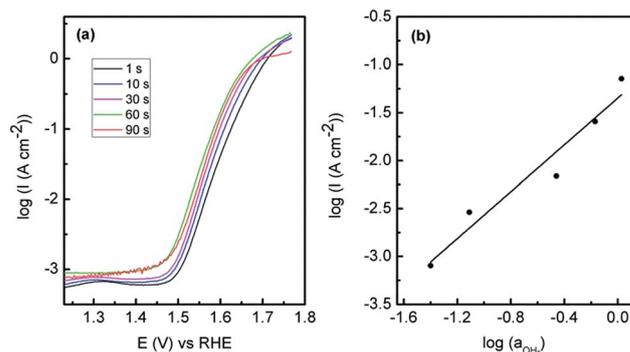
Fig. 7 (a) Tafel plots showing OER performance for  $\text{Au/Co(OH)}_2$  electrodeposited from  $10\text{ mM Co(NO}_3)_2 \cdot 6\text{H}_2\text{O}$  at different deposition time, (b) effect of hydroxide ion activity on OER. The cyclic voltammetric experiments used to obtain the data was recorded at a sweep rate of  $1\text{ mV s}^{-1}$  in  $1\text{ M NaOH}$ .
