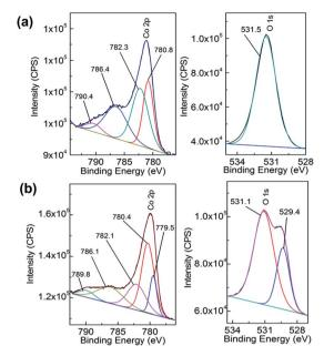
Fig. 3 XPS spectra of Co 2p (left panel) and O 1s (right panel) of (a) as deposited Co(OH)<sub>2</sub> on Au and (b) after 5 cycles into the OER region.
