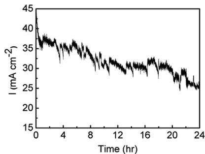
Fig. 9 Stability measurements of Au/Co(OH)<sub>2</sub> held at 1.67 V for 24 h in 1 M NaOH.
