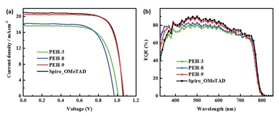
Fig. 5 (a) Current (J) –voltage (V) curves of the solar cells with PEH-3, PEH-8, PEH-9 and Spiro-OMeTAD control recorded from forward bias (FB) to short circuit conditions (SC) under AM 1.5 conditions (100 mW cm<sup>-2</sup>). (b) Incident photon-to-electron conversion efficiency (IPCE) as a function of wavelength for the PSCs in (a).
