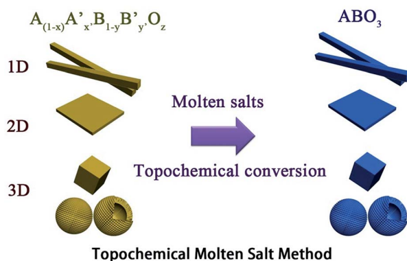
Fig. 1 The schematic illustration of the topochemical molten salt method.
