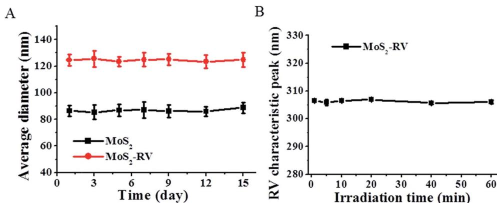
Fig. 5 (A) The average diameter changes of MoS<sub>2</sub> nanosheets and MoS<sub>2</sub>-RV, respectively in PBS buffer over 15 days. (B) The RV characteristic peak change of MoS<sub>2</sub>-RV under 808 nm laser irradiation (1 W cm<sup>-2</sup>) for different times. The data are shown as mean  $\pm$  S.D. ( $n = 4$ ).
