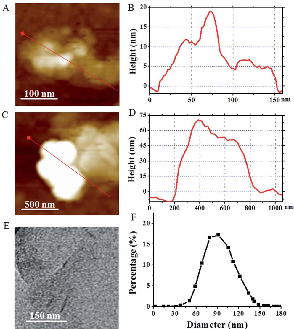
Fig. 2 (A and C) The AFM images of MoS<sub>2</sub> nanosheets (A) and bulk MoS<sub>2</sub> (C), respectively. (B–D) The corresponding AFM height analysis for MoS<sub>2</sub> nanosheets (B) and bulk MoS<sub>2</sub> (D), respectively. (E) The TEM image of MoS<sub>2</sub> nanosheets. (F) The size distribution of MoS<sub>2</sub> nanosheets as measured by DLS.
