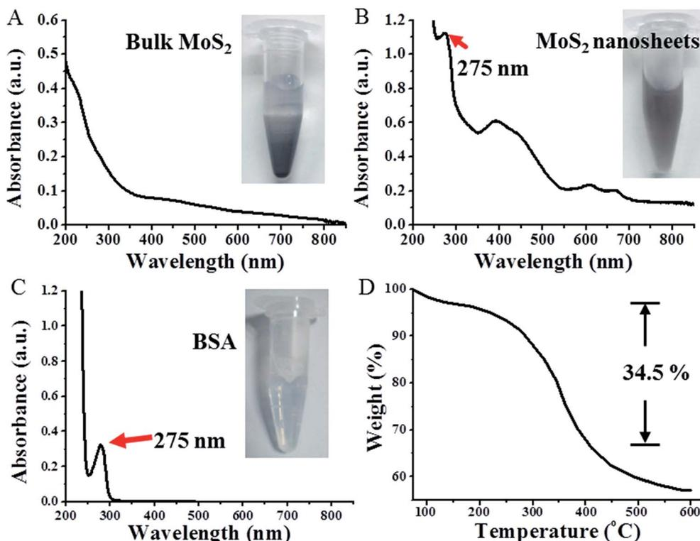
Fig. 3 The absorption spectra of bulk MoS<sub>2</sub> (A), MoS<sub>2</sub> nanosheets (B) and BSA (C), respectively. Insets are the corresponding images of bulk MoS<sub>2</sub> (A), MoS<sub>2</sub> nanosheets (B) and BSA (C) in aqueous solution, respectively. (D) TGA curve of MoS<sub>2</sub> nanosheets.
