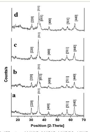
Fig. 3 XRD pattern of; [a] MNPs, [b] MS NPs, [c] MP (0.5 w/v%) NPs, and [d] MSP (0.5 w/v%) NPs. Magnetite Nanoparticles: MNPs; Magnetite/ Silica Nanoparticles: MS NPs; Magnetite/Pectin Nanoparticles: MP NPs and Magnetite/Silica/Pectin Nanoparticles: MSP NPs.
