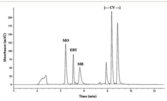
Fig. 1 HPLC chromatogram of model dyes: methyl orange (MO), Eriochrome black T (EBT), methylene blue (MB) and crystal violet (CV).
