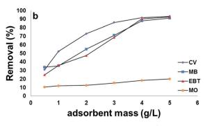
Fig. 9 Effect of adsorbent mass on the removal efficiency of model dyes onto: [a] MSP NPs and [b] MP NPs. Dyes  $100 \text{ mg L}^{-1}$ , temperature:  $25 \,^{\circ}\text{C}$ , pH: 2.0 for anionic dyes and 8.0 for cationic dyes, time: 120 min. Magnetite/Pectin Nanoparticles: MP NPs and Magnetite/Silica/Pectin Nanoparticles: MSP NPs.
