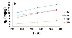
Fig. 10 Effect of temperature on the adsorption capacity ( $q_e$ ) of model dyes onto; [a] MSP NPs and [b] MP NPs. Adsorbent: 5 g L<sup>-1</sup>, dyes 10 mg L<sup>-1</sup>, pH: 2.0 for anionic dyes and 8.0 for cationic dyes, time: 120 min. Magnetite/Pectin Nanoparticles: MP NPs and Magnetite/Silica/Pectin Nanoparticles: MSP NPs.
