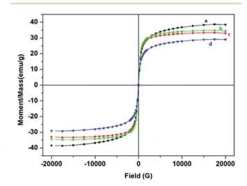
Fig. 5 Hysteresis loop of NPs of; [a] MNPs, [b] MS NPs, [c] MP NPs (0.5 w/v%) pectin, and [d] MSP NPs (0.5 w/v%) pectin. Magnetite Nanoparticles: MNPs; Magnetite/Silica Nanoparticles: MS NPs; Magnetite/Pectin Nanoparticles: MP NPs and Magnetite/Silica/Pectin Nanoparticles: MSP NPs.
