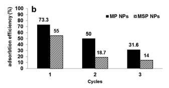
Fig. 11 Performance of magnetite/pectin NPs (MP NPs) and magnetite/silica/pectin NPs (MSP NPs) by three cycles of adsorption/desorption for [a] methylene blue and [b] Eriochrome black T.
