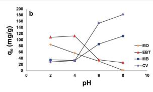
Fig. 12 Effect of pH on the adsorption capacity ( $q_e$ ) of model dyes in their mixture solutions onto; [a] MSP NPs and [b] MP NPs. Adsorbent: 2 g L<sup>-1</sup>, dyes 165 mg L<sup>-1</sup>, temperature: 25 °C, time: 120 min. Magnetite/Pectin Nanoparticles: MP NPs and Magnetite/Silica/Pectin Nanoparticles: MSP NPs.
