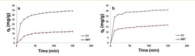
Fig. 7 Effect of contact time on the adsorption capacity ( $q_t$ ) of EBT and CV onto; [a] MSP NPs and [b] MP NPs. Adsorbent: 2 g L<sup>-1</sup>, dyes 100 mg L<sup>-1</sup>, temperature: 25 °C, pH: natural pH of dye, time: 150 min. Magnetite/Pectin Nanoparticles: MP NPs and Magnetite/Silica/Pectin Nanoparticles: MSP NPs.
