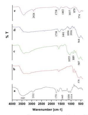
Fig. 4 FTIR data for; [a] pure pectin, [b] MNPs, [c] MS NPs, [d] MP (0.5 w/v%) NPs pectin, and [e] MSP (0.5 w/v%) NPs. Magnetite Nanoparticles: MNPs; Magnetite/Silica Nanoparticles: MS NPs; Magnetite/Pectin Nanoparticles: MP NPs and Magnetite/Silica/Pectin Nanoparticles: MSP NPs.
