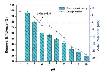
Fig. 5 Effect of initial solution pH values on  $Cr(v_i)$  removal by β-CCWB450 and zeta potential of β-CCWB450 at different solution pH.
