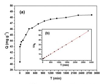
Fig. 6 Kinetics of Cr(vi) adsorption onto the  $\beta$ -CCWB450 at 298.15 K. (a) Cr(vi) sorption kinetics data, (b) pseudo-second-order model for Cr(vi) adsorption (initial Cr(vi) concentration 100 mg L $^{-1}$ ; pH = 2.0).
