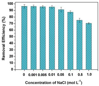
Fig. 9 Effect of different concentrations of NaCl on  $Cr(v_1)$  removal by  $\beta$ -CCWB450 ( $Cr(v_1)$  solution volume: 50 mL; adsorbent dose: 0.1 g; initial  $Cr(v_1)$  concentration: 100 mg  $L^{-1}$ ; contact time: 24 h; pH: 2.0).
