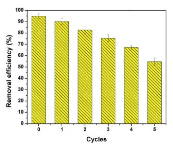
Fig. 10 Fifth consecutive adsorption–desorption cycles of  $\beta$ -CCWB450 for Cr(vı) removal (Cr(vı) solution volume: 50 mL; adsorbent dose: 0.1 g; initial Cr(vı) concentration: 100 mg L $^{-1}$ ; contact time: 24 h; pH: 2.0).
