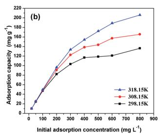
Fig. 4 (a) The comparison of adsorption capacity on  $\beta$ -CCWB and WB450 under 298.15 K, (b) the comparison of adsorption capacity on  $\beta$ -CCWB450 under different adsorption temperatures (Cr(vi) solution volume: 50 mL; adsorbent dose: 0.1 g; contact time: 24 h; pH: 2.0).
