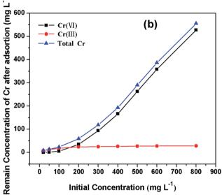
Fig. 11 (a) Time variation of Cr(III), Cr(VI) and total Cr concentration (initial Cr(VI) concentration: 100 mg  $L^{-1}$ ; Cr(VI) solution volume: 50 mL; adsorbent dose: 0.1 g; pH: 2.0), (b) initial concentration variation of Cr(IIII), Cr(VI) and total Cr concentration after adsorption (Cr(VI)) solution volume: 50 mL; contact time: 24 h; adsorbent dose: 0.1 g; pH: 2.0).
