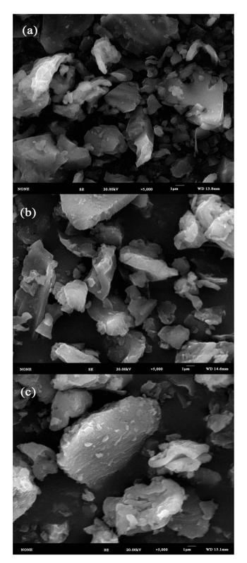
Fig. 1 SEM images of (a) pristine biochar, (b) modified biochar before adsorption and (c) after adsorption.
