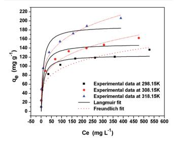
Fig. 7 Freundlich and Langmuir isotherms of  $Cr(v_1)$  adsorption on  $\beta$ -CCWB450 ( $Cr(v_1)$  solution volume: 50 mL; adsorbent dose: 0.1 g; contact time: 24 h; pH: 2.0).
