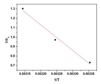
Fig. 8 Plot of  $\ln k^0$  versus  $T^{-1}$  for estimation of thermodynamic parameters for the adsorption of Cr(v<sub>I</sub>) on β-CCWB450 (Cr(v<sub>I</sub>) solution volume: 50 mL; adsorbent dose: 0.1 g; initial Cr(vI) concentration: 20, 50, 100, 200, 300, 400, 500, 600, 800 mg  $L^{-1}$ ; contact time: 24 h; pH: 2.0).
