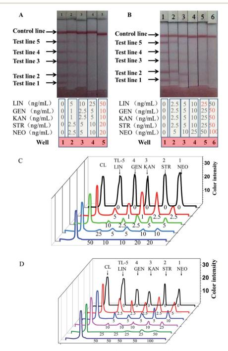
Fig. 4 Typical photo image of detection five analytes by the developed ICA in PBS (A) and milk (B) and optical density profiles of the test lines (TL-1, -2, -3, -4, and 5) and control lines (CL) of detection results in PBS (C) and milk (D).
