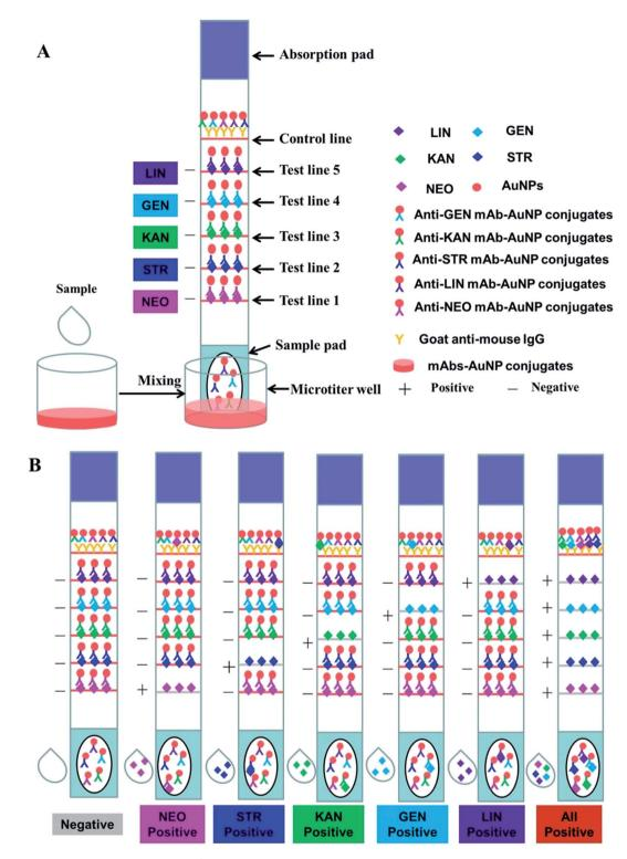
Fig. 1 Schematic illustration of the developed ICA.
