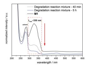
Fig. 4 UV-visible spectra illustrating the degradation of M1 in the presence of 5.5 equivalents of  $Na_2S_2O_4$  in a mixture of dichloromethane: methanol: water at reflux temperature (for details see section A.8 in the ESI†). Spectra recorded in THF at 25 °C.
