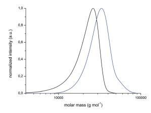
**Fig. 5** Molecular weight distribution of poly(MMA-*block*-CpCoCbMA) in THF (blue curve) obtained by sequential ATRP of the PMMA-Br macro-initiator (black curve) with CpCoCbMA **5**. The obtained values were calibrated against PS as standards.
