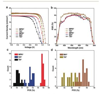
Fig. 4 (a) Photocurrent-voltage (J-V) characteristics, (b) EQE spectra and (c and d) statistical performance of the perovskite solar cells of different structures with various post-annealing treatments. a Represents the planar device and b represents the meso-structured device. A total of 100 cells (20 cells for each of post-annealing treatments) were considered for the statistical analysis. MPA-treated perovskite solar cells show improved efficiency compared to TA- and SA-treated PSCs.
