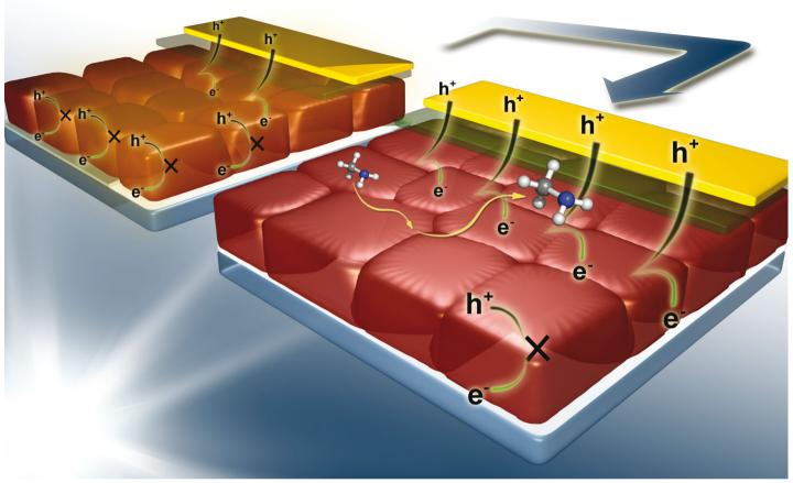
Showcasing the enhanced performance and stability of perovskite solar cells by methylamine post-annealing by Prof. Yabing Qi at the Energy Materials and Surface Sciences Unit (EMSS) in the Okinawa Institute of Science and Technology Graduate University (OIST).
