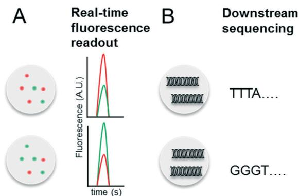
Fig. 4 Barcoding of droplets. (A) Optical encoding using two different fluorescence dyes (red and green) at different concentrations. This allows to encode for a maximum of  $x$  samples, with  $x = \text{number of dyes} \times \text{number of dye concentrations}$ . (B) Nucleotide sequence based barcoding. This allows to encode for a maximum of  $y$  samples, with  $y = 4^{(\text{number of nucleotides})}$ .
