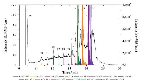
Fig. 3 RP-HPLC-ICP-MS/ESI-MS chromatograms obtained from clean-up fraction N showing all peaks detected by ICP-MS overlaid with extracted mass chromatograms detected by ESI-MS. The number of the peaks correspond to those listed in Table 1.
