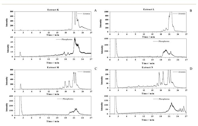
Fig. 2 RP-HPLC-ICP-MS for arsenic and phosphor chromatograms from cleaned fraction K (A), L (B), M (C) and N (D), using a mixture of chloroform/methanol with proportions of 2:1 (v/v), 1:1 (v/v); 1:2 (v/v) and methanol, respectively
