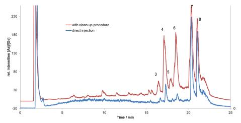
Fig. 6 HPLC-ICP-MS chromatogram of bentonite (2 g of sample) extracted from of 5 mL of methanol, shaking for 2 min and immediately injected without clean-up in RP-HPLC-ICP-MS, compared to the methanol fraction after clean up (extract N). The number of the peaks are the same as in Fig. 3.
