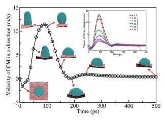
Fig. 5 Gold film CM velocity profile in the z direction along with the snapshots of MD simulation performed at 1073 K. The diameter and thickness of the film are 30 nm and 10 Å. Inset shows the velocity of the CM for different thicknesses of film.
