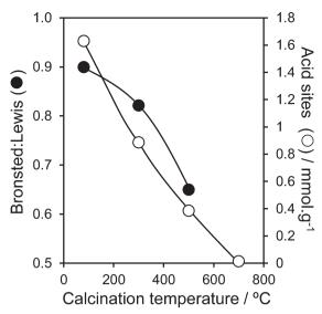
Fig. 2 Brønsted: Lewis character and total acid site density of PNA as a function of calcination temperature.
