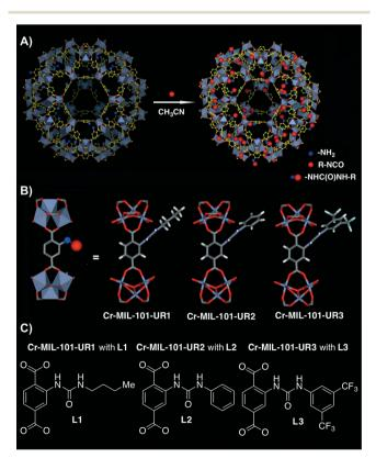
Fig. 4 A) PSM approach of  $Cr-MIL-101-NH_2$  with isocyanates to generate Cr-MIL-101-UR1-3. B) Schematic representation of the ligand structure and  $[Cr_3O(CO_2)_6]$  cluster nodes. C) Differently substituted ureas present in the final synthesised MOFs. Adapted with permission from ref. 50. Copyright ® Royal Society of Chemistry.
