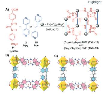
Scheme 5 A) Synthesis of catalytic urea-containing MOFs TMU-18 (triclinic  $P\bar{1}$ ) and TMU-19 (orthorhombic Pnna). B) and C) View along the pore direction of TMU-18 and TMU-19, respectively. In contrast to TMU-18, TGA analysis indicated a lower thermal stability for TMU-19. Adapted with permission from ref. 53. Copyright ® Royal Society of Chemistry.
