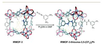
7 PSM IRMOF-3 between with approach bis(trifluoromethyl)phenyl isothiocyanate. Adapted with permission from ref. 56. Copyright ® Royal Society of Chemistry.
