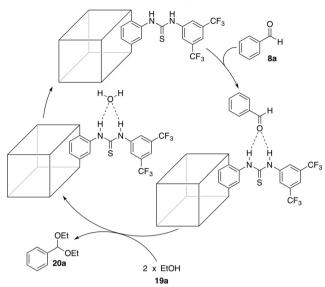
Scheme 8 Mechanistic proposal for the acetalisation reaction catalysed by IRMOF-3-thiourea-3,5-(CF<sub>3</sub>)<sub>2</sub>Ph.<sup>56</sup>
