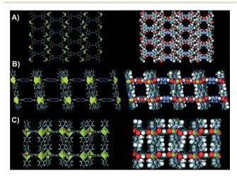
Fig. 2 Stick and space-filling representations of NU-601 (P2<sub>1</sub>/c space group). A) View down the a axis (pore size 12.05 Å imes 13.95 Å). B) View down the b axis (pore size 11.38 Å  $\times$  13.69 Å). C) View down the c axis (pore size 11.38 Å  $\times$  4.87 Å). Adapted with permission from ref. 43. Copyright ® American Chemical Society.
