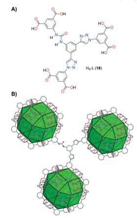
Fig. 6 A) Structure of the hexacarboxylate acid H<sub>6</sub>-L (18). B) Single crystal structure of the (3,24)-connected rht-topological framework in Cu-UBTA. Tetragonal space group I4/m, unit cell dimensions a = b = 131.4206 Å, c = 44.8239 Å. BET surface area = 3134 m<sup>2</sup> g<sup>-1</sup>. Adapted with permission from ref. 55. Copyright ® Royal Society of Chemistry.
