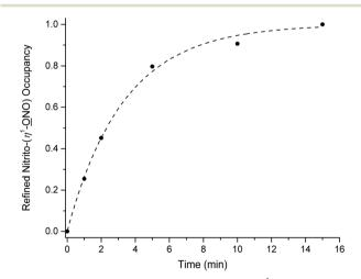
Fig. 3 Plot of crystallographically-refined nitrito-(η¹-QNO) occupancy vs. irradiation time (excitation at  $\lambda = 400$  nm) for steady-state photocrystallographic experiments with (1) between 0 and 15 min illumination. JMAK kinetic analysis:  $k = 0.30(2) \text{ min}^{-1}$ , (0.0049(3) s<sup>-1</sup>),  $n = 0.30(2) \text{ min}^{-1}$  $0.98(7), R^2 = 0.99.$
