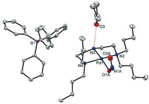
Fig. 4 Single-crystal X-ray structure for the asymmetric unit of (1) showing the atomic arrangement in the metastable state (MS) after 1 h irradiation at  $\lambda$  = 400 nm. Ellipsoids set at 50% probability and hydrogen atoms omitted for clarity (red dashed line = hydrogen bonding to THE solvent molecule)
