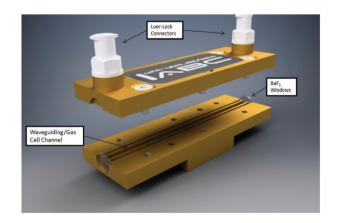
Fig. 2 CAD models of a custom 75 mm long straight-channel iHWG (channel cross-section: 4 mm $^2$ ) equipped with Luer-Lock connectors for gas in/out, and IR-transparent BaF $_2$  windows sealing the hollow channel for efficient IR radiation in/out coupling.
