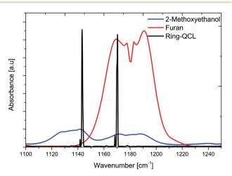
**Fig. 4** Laser emission lines (black) overlaid with the IR spectrum of furan (red), and 2-methoxyethanol (blue). The emission spectrum of the riQCL was obtained by coupling the emitted laser radiation into a Fourier transform infrared (FT-IR) spectrometer.
