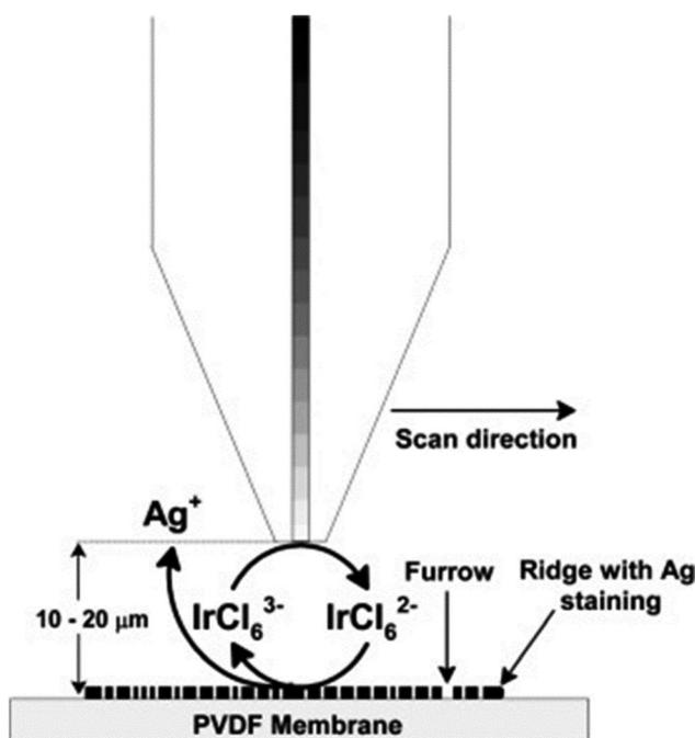
Fig. 13 Schematic (not to scale) of the operating principle for SECM imaging of silver stained fingerprints on the PVDF membrane using  $\text{IrCl}_6^{3-}$  oxidation ( $E_{\text{tip}} = 0.8 \text{ V vs. Ag QRE}$ ) at the tip.<sup>99</sup> Reproduced from ref. 99 with permission from the Elsevier.
