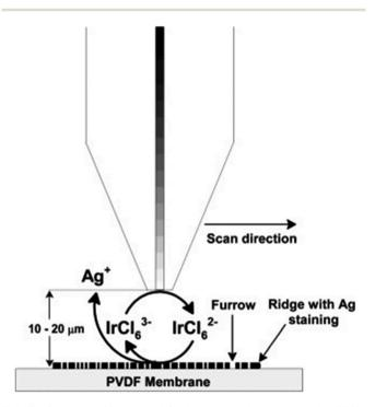
**Fig. 13** Schematic (not to scale) of the operating principle for SECM imaging of silver stained fingermarks on the PVDF membrane using  ${\rm IrCl_6}^{3-}$  oxidation (Etip = 0.8 V vs. Ag QRE) at the tip. <sup>99</sup> Reproduced from ref. 99 with permission from the Elsevier.
