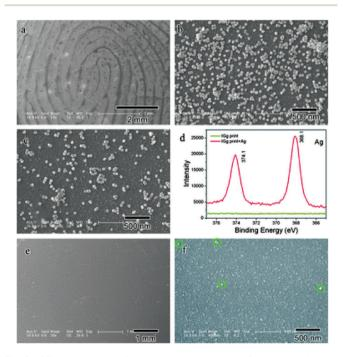
Fig. 2 SEM images of a fingermark with human IgG incubated by the ASNRPC: (a) with a lower and (b) higher magnification on the ridges and (c) beside the ridges; (d) XPS spectra of the fingermark with human IgG before and after incubation with the ASNRPC; SEM images of the fingermark with human IgG before incubation with the ASNRPC: (e) with a lower and (f) higher magnification. 31 Reproduced from ref. 31 with permission from the Royal Society of Chemistry.
