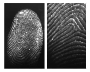
**Fig. 11** A charged latent fingermark on a PVDF substrate developed by using the aptamer-based reagent. The fingermark was aged for 24 hours before it was developed with the lysozyme aptamer 1 reagent containing CAL Fluor® Orange 560 as the fluorescent tag. 91 Reproduced from ref. 91 with permission from Wiley.
