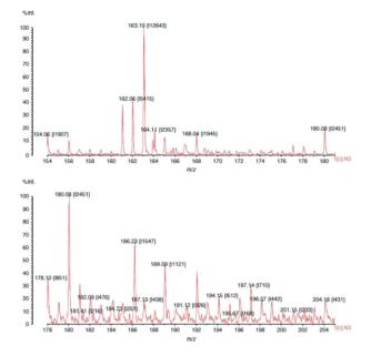
Fig. 4 SALDI-MS plot of a smoker's fingermark showing a nicotine peak at m/z 163. The print was dusted using hydrophobic silica powder and lifted with a conductive adhesive tape. 40 Reproduced from ref. 40 with permission from Wiley.
