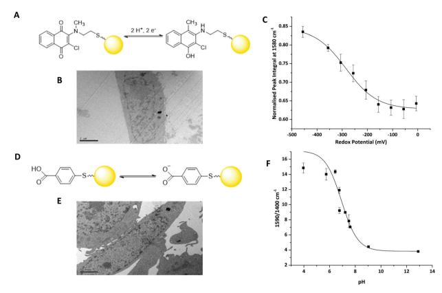
Fig. 2 (A) Structure and equilibrium between oxidised and reduced forms of MeNQ·NS (yellow sphere represents gold NS, not to scale). (B) TEM image of MeNQ·NS in the cytoplasm of a PC3 cell. (C) Calibration curve for MeNQ·NS (D) Equilibrium between protonated and deprotonated forms of pMBA·NS. (E) TEM image of pMBA·NS in the cytoplasm of a PC3 cell. (F) Peak height calibration curve for pMBA·NS.
