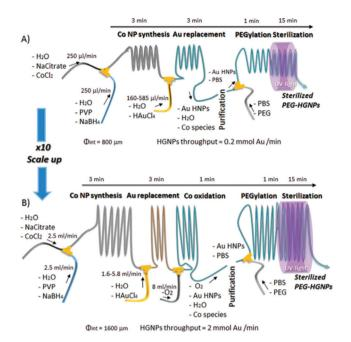
Fig. 2 Experimental set up for the production of HGNPs produced from galvanic replacement of sacrificial Co templates, including stages PEG functionalisation and sterilisation on a singular platform, scaled up for high throughput. Reprinted with permission from L. Gomez, V. Sebastian, S. Irusta, A. Ibarra, M. Arruebo and J. Santamaria, Lab Chip, 2014, 14, 325-332. Copyright (2014) Lab Chip.
