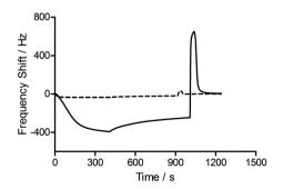
Fig. 4 Frequency responses of protein binding and sensor surface regeneration. Anti-biotin  $F_{ab}$  binding to biotin-derivatized pAAc surface (–); anti-biotin  $F_{ab}$  binding to biotin-derivatized carboxyl-terminated SAM surface (---). Sample concentrations: 25  $\mu$ g mL<sup>-1</sup>; flow rate: 25  $\mu$ L min<sup>-1</sup>. Surfaces were regenerated with glycine (10 mM, pH 1.5).
