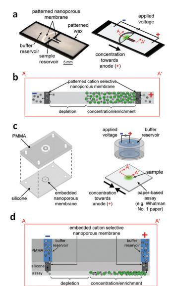
Fig. 3 Design and operation of the external and in-paper devices for concentration. (a) Schematic of the in-paper transport configuration. (b) Cross-section of the in-paper devices illustrating ICP under an applied voltage. (c) Schematic of the external concentration device. (d) Crosssection of the devices and paper-based assays depicting ICP under an applied voltage. (Image reproduced from ref. 11 with permission. Copyright 2016, American Chemical Society.)
