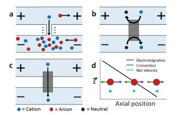
Scheme 1 Illustration of (a) ICP, (b, c) FICP, and (d) ICP CFF mechanisms.
