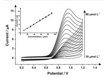
Fig. 4 Cyclic voltammograms obtained from additions of sodium nitrite (10–90  $\mu$ mol L $^{-1}$ ) into pH 7 PB using a 3 minute mechanical activation/polished SPE with alumina slurry using the same SPE throughout the experimentation (scan rate: 100 mV s<sup>-1</sup> vs. SCE); the dotted line represents the blank (no sodium nitrite) response. Inset: analysis of the voltammetric peak heights as a function of concentration.
