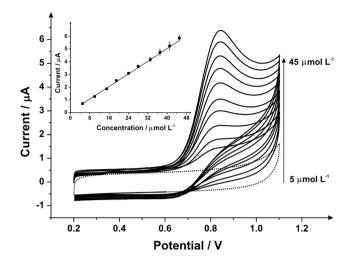
Fig. 7 Cyclic voltammograms obtained from additions of sodium nitrite (5-45 µmol L<sup>-1</sup>) into pH 7 PB using a 1 minute mechanically activated/ polished SPE with diamond slurry using the same SPE throughout the experimentation (scan rate: 100 mV s<sup>-1</sup> vs. SCE); the dotted line represents the blank (no sodium nitrite) response. Inset: analysis of the voltammetric peak heights as a function of concentration.
