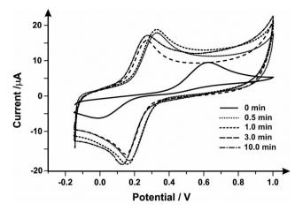
Fig. 1 Cyclic voltammetric responses obtained using a SPE in 1 mmol L<sup>-1</sup> ammonium iron(||) sulfate/0.2 M HClO<sub>4</sub> solution as a result of varying mechanical activation/polishing times using alumina slurry. Scan rate: 50 mV s<sup>-1</sup> vs. SCE.
