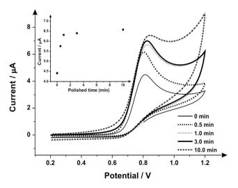
Fig. 3 Cyclic voltammetric study of the variation of mechanical activation/polishing times recorded in 50 µmol L<sup>-1</sup> sodium nitrite/PBS (pH 7) using SPEs (different SPE per experiment). Inset: a plot of current as a function of mechanical activation/polishing time (with alumina slurry) variation. Scan rate: 50 mV s<sup>-1</sup> vs. SCE.
