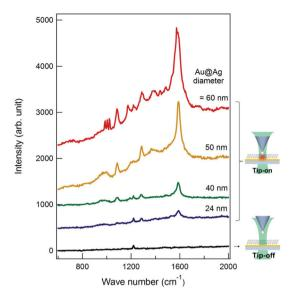
Fig. 4 A set of BPT TERS spectra with (tip-on, colored lines) and without (tip-off, black line) Au@Ag NP-tips. The same BPT sample was used for all of the measurements. Each spectrum was obtained with a laser power of 20  $\mu$ W, and the integration time was 180 s. For the ease of viewing, each of the spectra is vertically offset.
