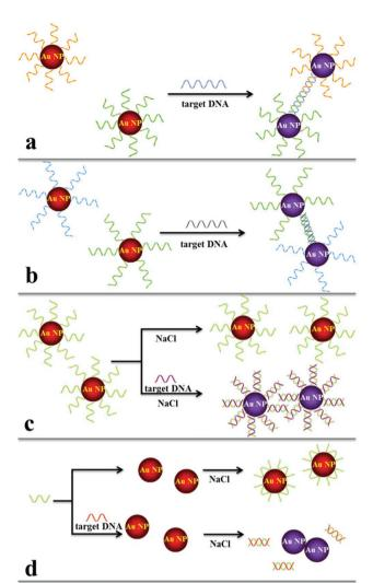
**Fig. 1** Schematics of colorimetric DNA hybridization detection systems. Duplex (a) and triplex (b) DNA crosslinking and non-crosslinking of (c) thiolated DNA–Au NPs and (d) non-thiolated DNA and Au NP.
