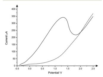
**Fig. 1** Linear sweep voltammograms using CuSPEs in the absence (dashed line) and presence of 1 mM sulfide (solid line) in pH 8 B–R buffer solution. Deposition time and potential of 60 s at -0.4 V respectively (vs. Ag/AgCl) and scan rate 100 mV s<sup>-1</sup>.
