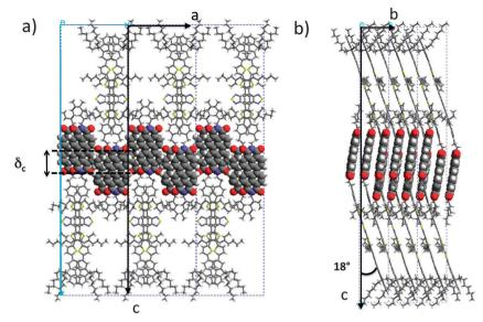
Fig. 5 Projections of the refined structural model of AD<sub>0</sub> yielding the calculated diffraction patterns in Fig. 4. The projections are along the b axis (a) and along the a axis (b)
