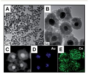
Fig. 2 TEM (A and B), and HAADF-STEM images (C to E) of Au@CeO<sub>2</sub>.
