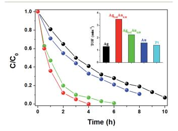
Fig. 3 Catalytic reduction of 4-NP by Ag@CeO2 (black), Ag0.64- $Au_{0.36}$ @CeO<sub>2</sub> (red),  $Ag_{0.41}$ Au<sub>0.59</sub>@CeO<sub>2</sub> (green) and Au@CeO<sub>2</sub> (blue). Inset: calculated TOF compared with Pt@CeO<sub>2</sub>.7
