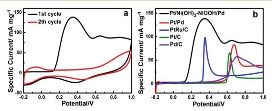
Fig. 4 (a) CO stripping voltammograms on the Pt/Ni(OH) $_2$ -NiOOH/Pd MHNRAs performed in a solution of 0.5 M H $_2$ SO $_4$  at 20 mV s $^{-1}$ ; (b) the comparison of the CO stripping voltammograms of the Pt/Ni(OH) $_2$ -NiOOH/Pd MHNRAs, Pt/Pd MHNRAs, commercial Pt/C, Pd/C and PtRu/C catalysts.
