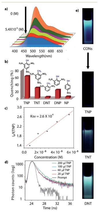
Fig. 5 (a) Turn off sensing (PL quenching); (b) degree of fluorescence quenching of TfpBDH-CONs with analytes; (c) Stern–Volmer plots for the quenching of CONs by TNP; (d) fluorescence decay profile ( $\lambda_{\rm ex}=365$  nm and  $\lambda_{\rm em}=447$  nm) of TfpBDH-CONs, in the presence of different analytes; (e) digital photographs of the turn off sensing of analytes under UV light ( $\lambda_{\rm ex}=365$  nm).
