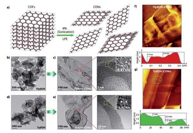
Fig. 4 (a) Schematic representation of COFs to CONs formation; HR-TEM images of (b and d) TfpBDH and TpBDH; and (c and e) TfpBDH-CONs and TpBDH-CONs; (f and q) AFM images of TfpBDH-CONs and TpBDH-CONs with corresponding height profiles (the height profiles, colourfilled red and green, are measured along the corresponding tracks inside the circle shown in the AFM images).
