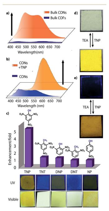
Fig. 6 (a) Photoluminescent spectra of bulk TfpBDH and TfpBDH-CONs; (b) photoluminescent spectra showing turn on (PL enhancement) of bulk TfpBDH-CONs and with TNP; (c) photoluminescence enhancement plots of different analytes [at  $5.4 \times 10^{-3}$  (M)] with TfpBDH-CONs; (d and e) solid state sensing (turn on) by TfpBDH-CONs in presence of TNP under visible and UV light (365 nm) which also exhibits the reversible color change from blue to yellow and *vice versa* upon TEA treatment.
