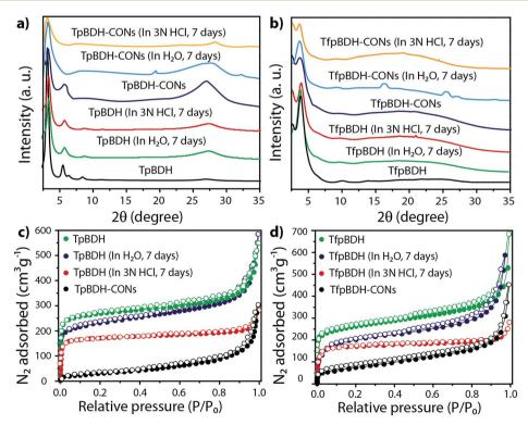
Fig. 3 (a and b) PXRD patterns before and after chemical stability tests of TpBDH, TpBDH-CONs; TfpBDH, and TfpBDH-CONs respectively; (c and d)  $N_2$  sorption isotherms; shows the chemical stability of TpBDH, TfpBDH in water and 3 N HCl for 7 days.
