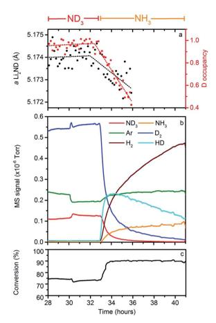
Fig. 7 H-D exchange experiment, where the gas species flowing across the sample during the experiment are shown at the top. The panels show (a) the refined deuterium occupancy (red) and lattice parameter (black) in the Li<sub>2</sub>ND sample, (b) the QGA data collected during the experiment and (c) the ammonia conversion percentage data
