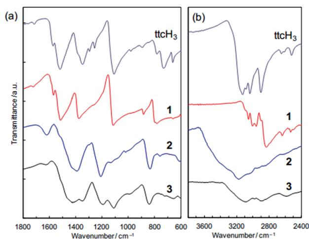
Fig. 4 FTIR spectra of 1, 2 and 3 compared with pure trithiocyanuric acid. (a) 600–1800 cm<sup>-1</sup>. (b) 2400–3800 cm<sup>-1</sup>.
