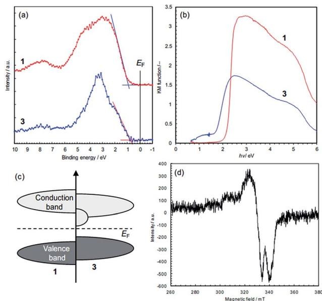
Fig. 7 Spectroscopic data of the frontier orbitals in **1** and **3**. (a) XPS data of valence bands. The valence band maxima were obtained by extrapolation of the onset linear parts: 1.0 eV for **1** and 0.8 eV for **3**. (b) Kubelka–Munk functions obtained by diffuse reflectance spectroscopy. (c) Schematic illustration of the positions of the frontier orbitals. (d) X-band ESR spectra for Cu(II) ions in **3**.
