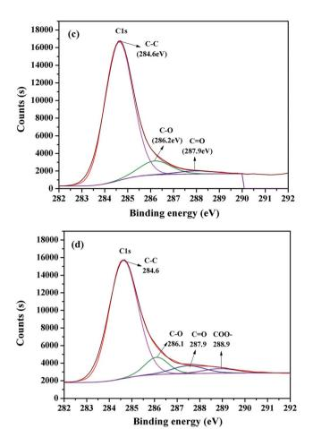
Fig. 3 C 1s XPS spectra of biochar (c) before and (d) after modification.
