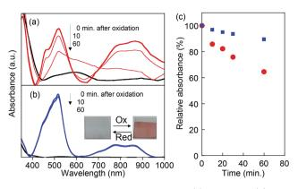
Fig. 3 In situ electrochemical UV spectra of (a) PVBPT and (b) PVPPP on ITO electrode. A neutral phenothiazine form was shown in black, and the corresponding radical cations under the applied potentials at 1.1 V were shown in red and blue, respectively. (c) Time decay of the relative absorbance at 518 nm ascribed to the radical cations for PVBPT (red) and PVPPP (blue).
