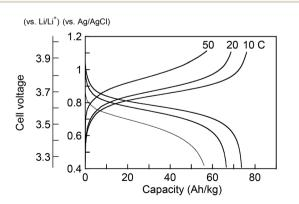
**Fig. 4** Charge–discharge curves of PVPPP composite electrodes on glassy carbon.
