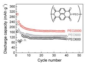
Fig. 10 Discharge capacities *versus* cycle number for naphthalene polyimide-b-PEO600 ( $\bigcirc$ ), naphthalene polyimide-b-PEO900 ( $\triangle$ ) and naphthalene polyimide-b-PEO2000 ( $\square$ ) at  $1Li^+/5$  h rate.
