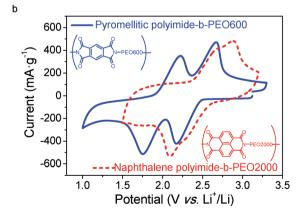
Fig. 7 (a) Redox reaction of pyromellitic and naphthalene polyimides. (b) Cyclic voltammograms of an electrode containing pyromellitic polyimide-b-PEO600 (solid blue) and naphthalene polyimide-b-PEO600 (dashed red) in 1 M LiTFSI/MeTHF. Scan rate: 1 mV s<sup>-1</sup> Normalized current per gram of redox-active material.
