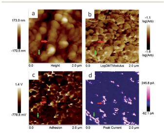
Fig. 6 AFM images collected in the PeakForce TUNA mode, using a DC sample bias of 1 V on sample naphthalene polyimide-b-PEO600 loaded with 15 wt% of carbon black. (a) Topography, (b) elastic modulus in log scale, (c) adhesion force and (d) peak current images. The red and green arrows are pointing on the same domains in all four pictures
