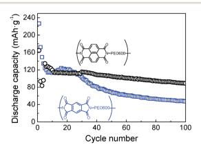
Fig. 8 Discharge capacities *versus* cycle number for pyromellitic polyimide-b-PEO600 ( $\square$ ) and naphthalene polyimide-b-PEO600 ( $\bigcirc$ ) at 1Li<sup>+</sup>/5 h rate.
