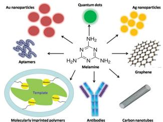
Fig. 1 Novel recognition and transducer components used for the fabrication of sensors for melamine determination.
