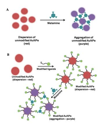
Fig. 2 Schematic presentation of the colorimetric mechanism for melamine determination employing unmodified AuNPs (A) and modified AuNPs (B).
